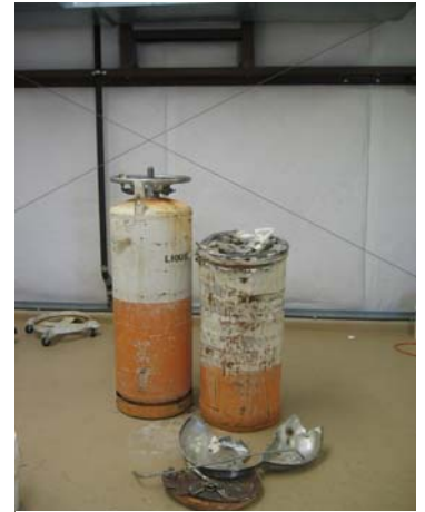
Figure 1 -Effect of Explosion on Dewar Cylinder Compared to unaffected cylinder
