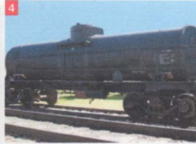
Examples of aging equipment: 2. Silos 3. Separation equipment 4. A riveted tank car
